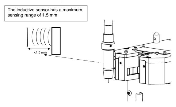
When a nozzle is detected by the sensor, the "Nozzle Detect" input will turn on and the "Ready" signal will turn off.
