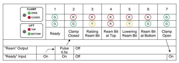
The above chart shows the robot inputs and outputs as the sequence progresses.
