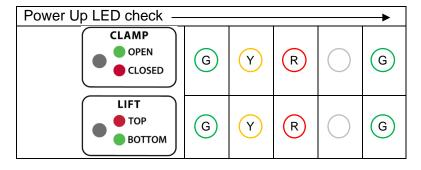
If the sensor LEDs are not reporting the clamp open and the lift at the bottom, then check the air pressure or sensor positions. If the sensor LEDs are flashing yellow and green, check for **start lock** (see below). If the LEDs are flashing yellow, ensure the settings pushbutton is not pressed or defective.
